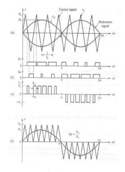
Figure 5: Sinusoidal PWM
