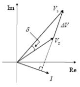
Figure 3: Vector Diagram of Power Transmission Based on Two AC Voltage Sources Interconnected through a Lossless Reactor
